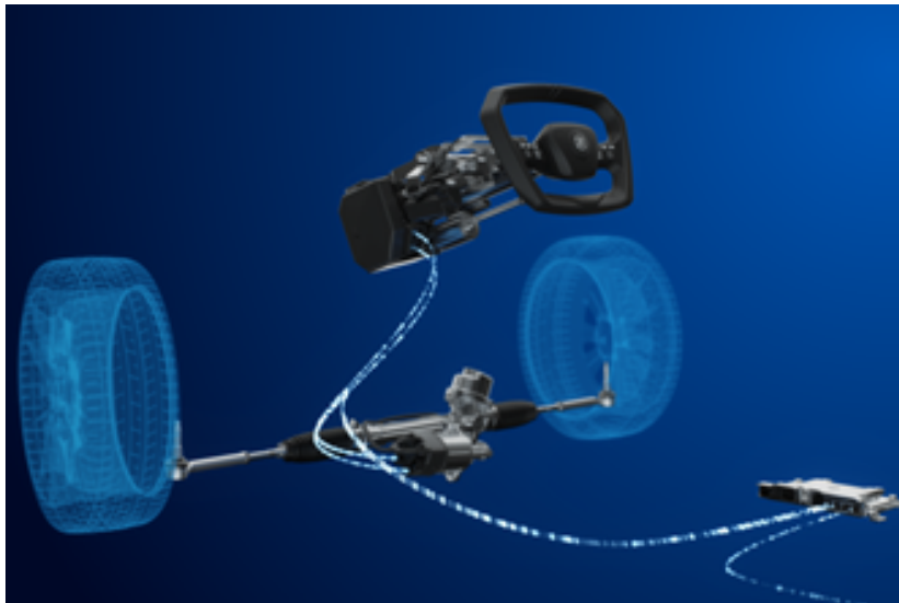
Figure 13 Steer-by-wire concept Source
