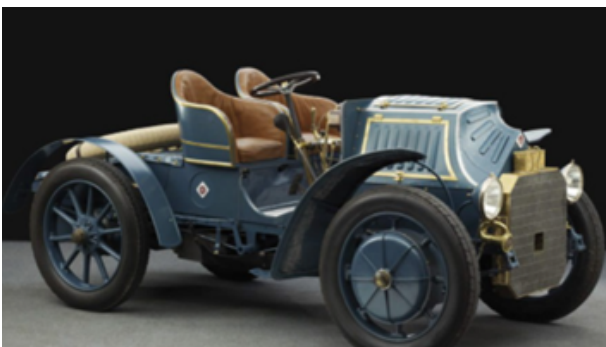
Fig. 6. The Lohner-Porsche Mixte, the first commercially available hybrid car
